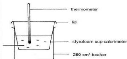
1. Set up equipment and Fill the beaker with cotton wool to help insulate so that less heat loss (with lid) to surroundings.
